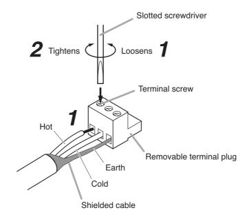
**Tip**Recommended slotted screwdriver type: Screwdriver with blade that is 3 mm in width
